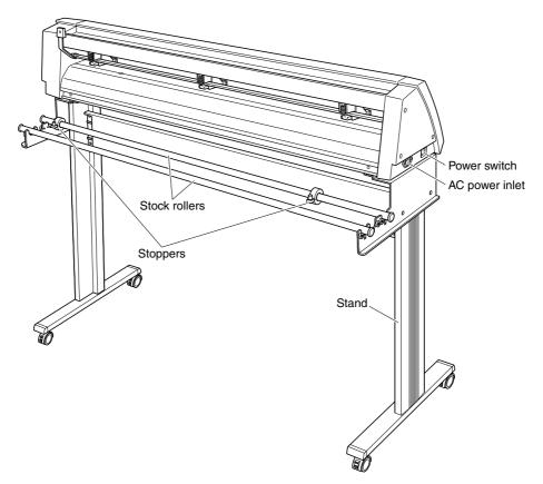
AC power inlet Power switch Stand Stock rollers Stoppers
