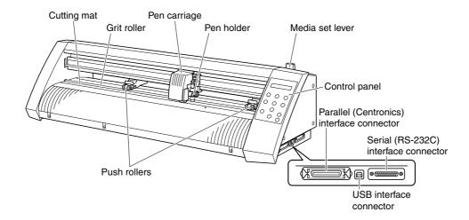
Cutting mat: Cutting or plotting is performed on this mat.Grit roller: Feeds the medium backward or forwardPush rollers: Pushes the medium against the grit rollersPen carriage: Moves the cutter pen to the left and rightPen holder: Holds the cutter pen and moves it up and down
