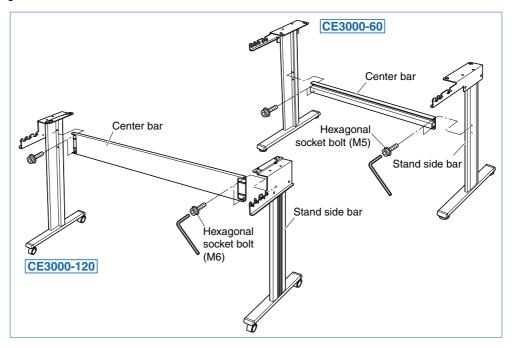
Mount the CE3000 cutting plotter on the stand by inserting the positioning pins on the stand into the positioning holes on the underside of the cutting plotter. Fasten using the four coin screws or hexagonal socket bolts (M6).
