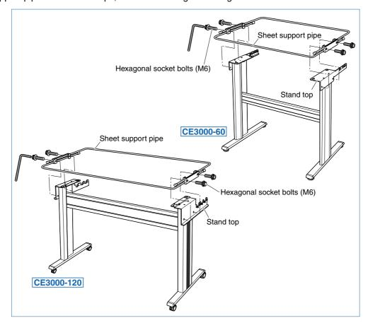
Mount the CE3000 cutting plotter on the stand by inserting the positioning pins on the stand into the positioning holes on the underside of the cutting plotter. Fasten using the four coin screws or hexagonal socket bolts (M6).
