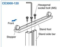
Fasten the stand tops (L/R) to the stand side bars (L/R) with the hexagonal socket bolts (M5), using the Allen wrench.
